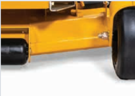
Commercial-Grade Deck 10 ga. with front bull nose bumper
